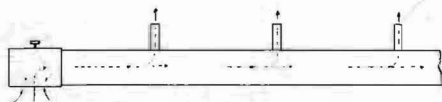
Fig. 2 Air flow in a ventilation system having an extended plenum supply duct.
