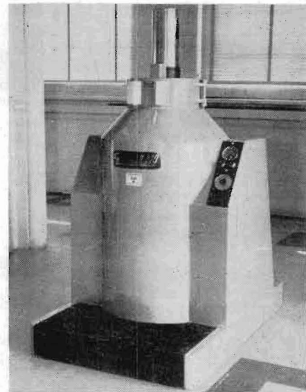
Cobalt 60 gamma irradiator "Gammacell 220" with built-in shielding can be installed in any laboratory for radiation research. Controls in panel on right permit automatic exposure of samples for pre-set periods to gamma radiation from the shielded Cobalt 60 source. (Photograph—Courtesy, Commercial Products Division, Atomic Energy of Canada Limited.)
