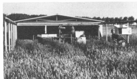
Figure 1. Lysimeter installation at the Lethbridge Research Station showing weighing equipment, gantry, and automatic rain shelter.
