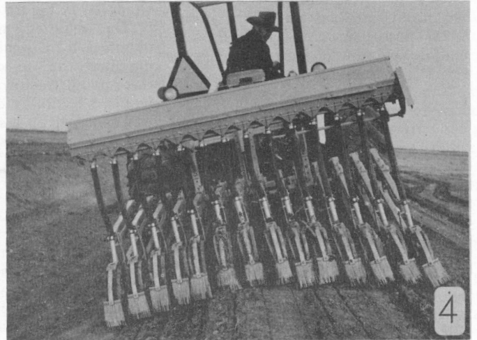
Figure 1. Grass seeder in transport position. Note parallel-arm suspension and the movable stops for adjusting the spring pressure on each opener. Figure 2. Grass seeder mounted on three-point hitch of tractor seeding the ditch bank. Figure 3. Grass seeder mounted on three-point hitch of tractor seeding the bottom of the ditch. Figure 4. Seeder equipped with plastic brushes seeding a packed ditch bank.
