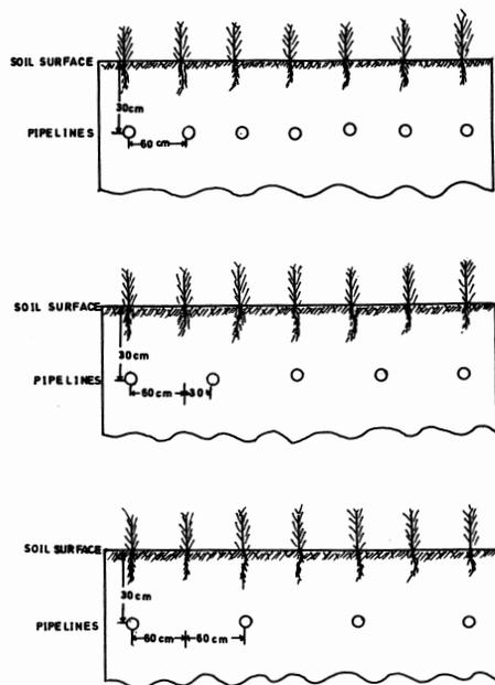
Figure 1. A sketch showing the layout of pipe lines and the crop rows at the various subsurface irrigation spacings.
