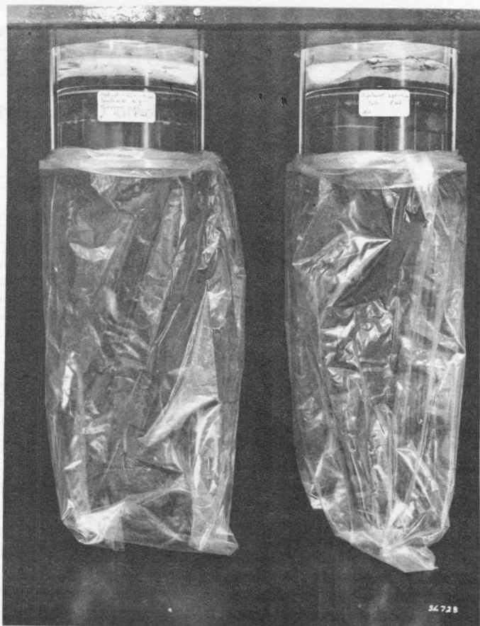
Figure 1. Soil-asphalt discs being subjected to seepage control testing. The discs are located at the label level in the cylinders and the plastic bags are to catch any effluent should there be seepage.
