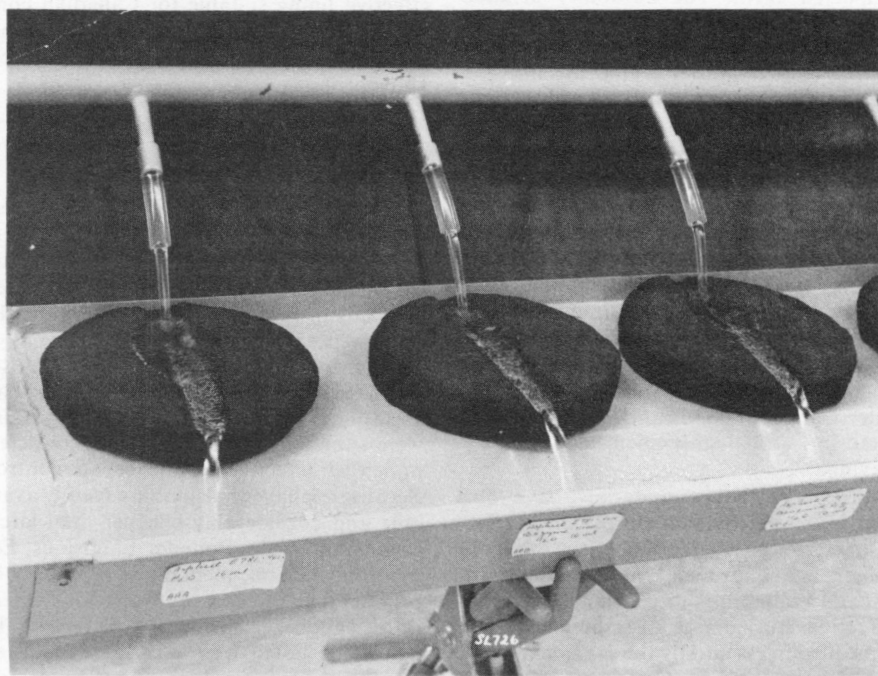
Figure 2. Small stream of water flowing over soil-asphalt discs (on a 25% slope).
