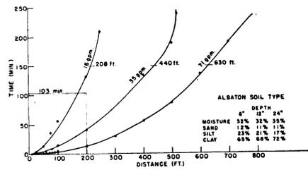
Figure 3. Rate-of-advance curves for Albaton soil type.
