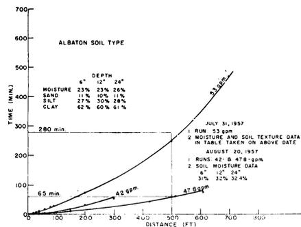
Figure 6. Rate of advance curves for Albaton soil type.
