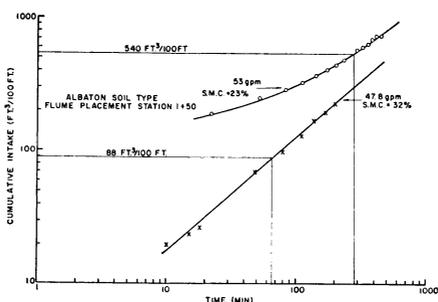
Figure 7. Mass intake characteristics of Albaton soil.
