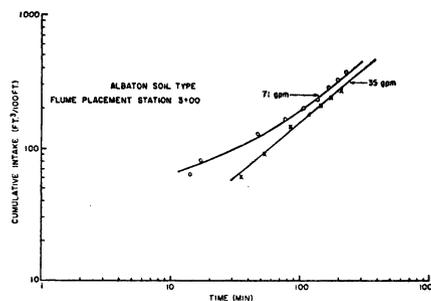
Figure 4.—Mass-intake characteristics of Albaton soil.
