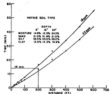
Figure 5. Rate of advance curves for Haynie soil type.
