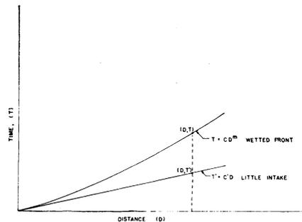
Figure 1. Estimation of furrow intake rate (1)
