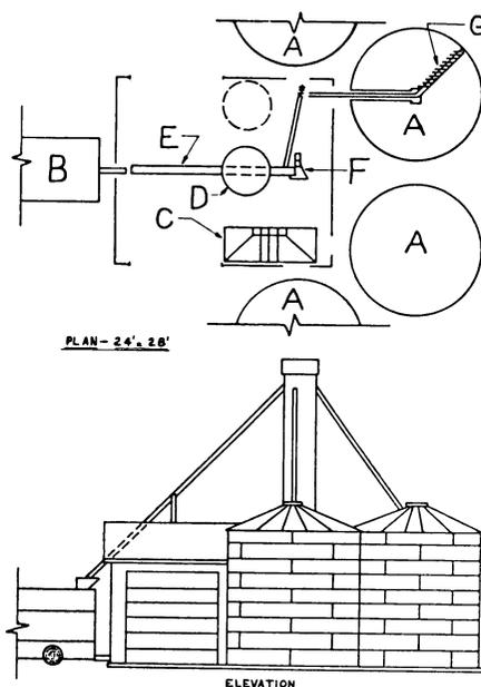
Figure 4. A grain-feed handling system for shelled grain. A—18' Dia. 3000 bu. bins, B—Dryer, C—Automatic grinder mixer with hopper bin, D—Wet Corn or Bulk Supplement, E—Belt, F—Bucket elevator, C—Unloader.
