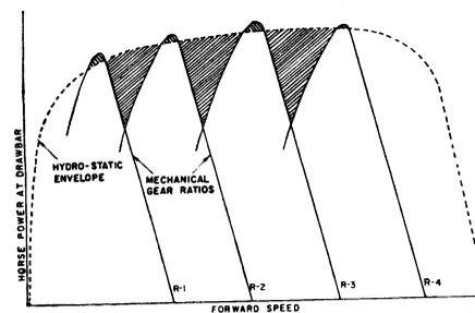
Figure 3. Gear transmission compared to hydrostatic system
