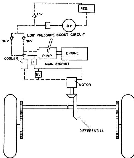
Figure 2. Hydrostatic system with conventional axle and gear reduction.
