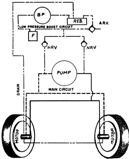
Figure 1. Hydrostatic tractor system with slow-speed motors at wheels.
