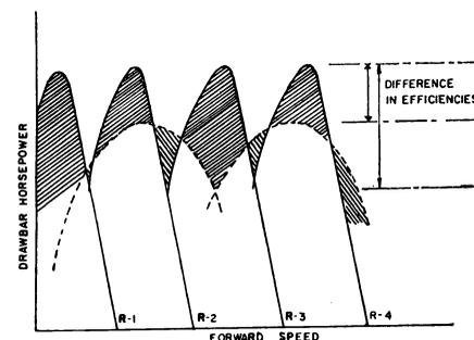
Figure 4. 4-gear mechanical compared to 2-gear torque converter system.
