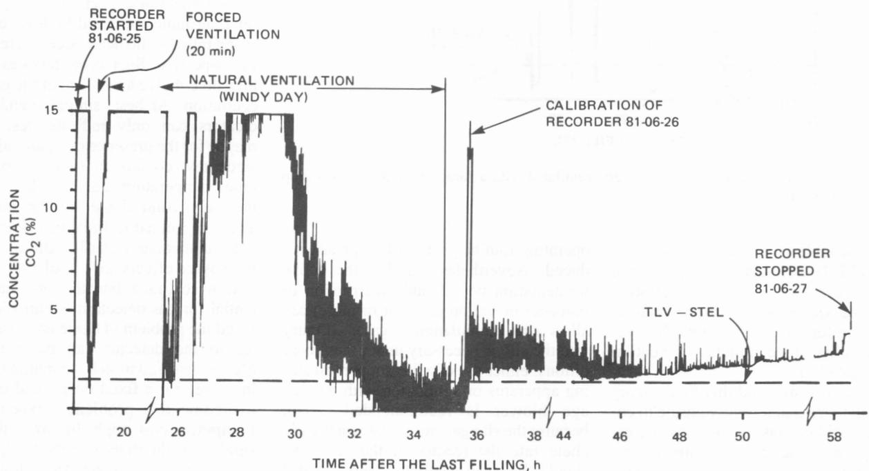
Figure 7. Recorder chart for  $\text{CO}_2$ , silo 23, 1981.
