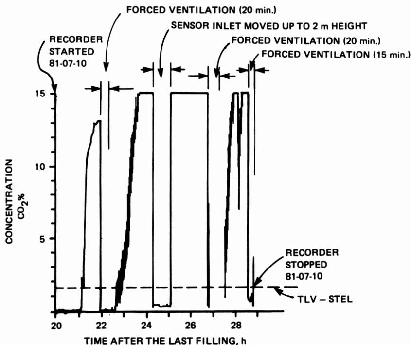
Figure 9. Recorder chart for CO<sub>2</sub> in silo 26, ventilated with a forage blower and 5-m drop tube, 1981.
