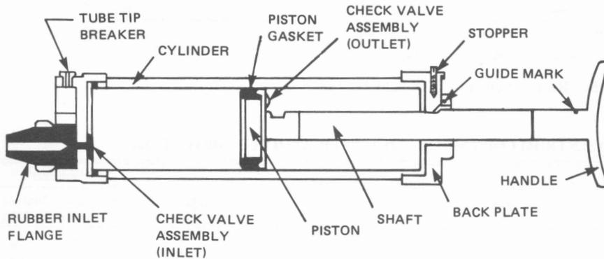
Figure 3. Piston and cylinder type gas detection pump (Gastec).
