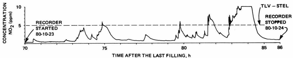
Figure 5. Recorder chart for NO<sub>2</sub>, silo 21, 1980.
