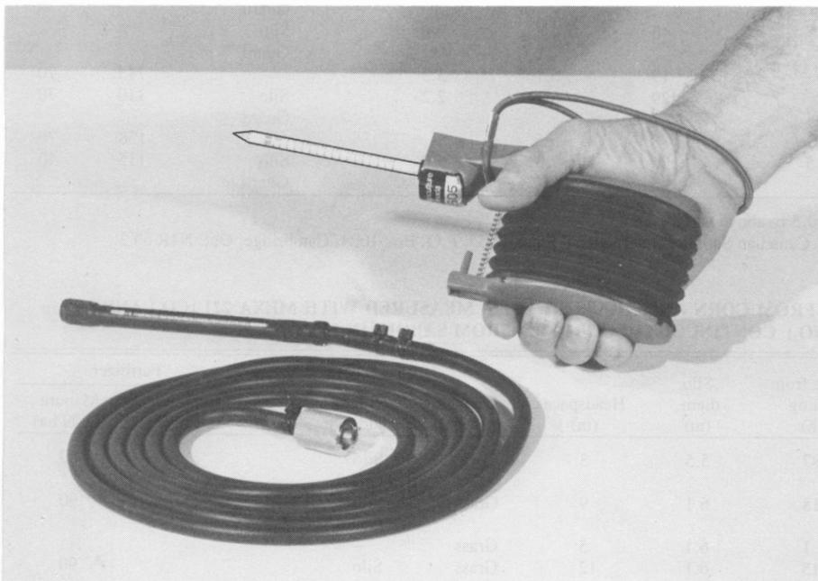
Figure 4. Dräger gas tester consisting of bellows pump, attached chemical tube and 5.5-m extension hose for remote sampling.
