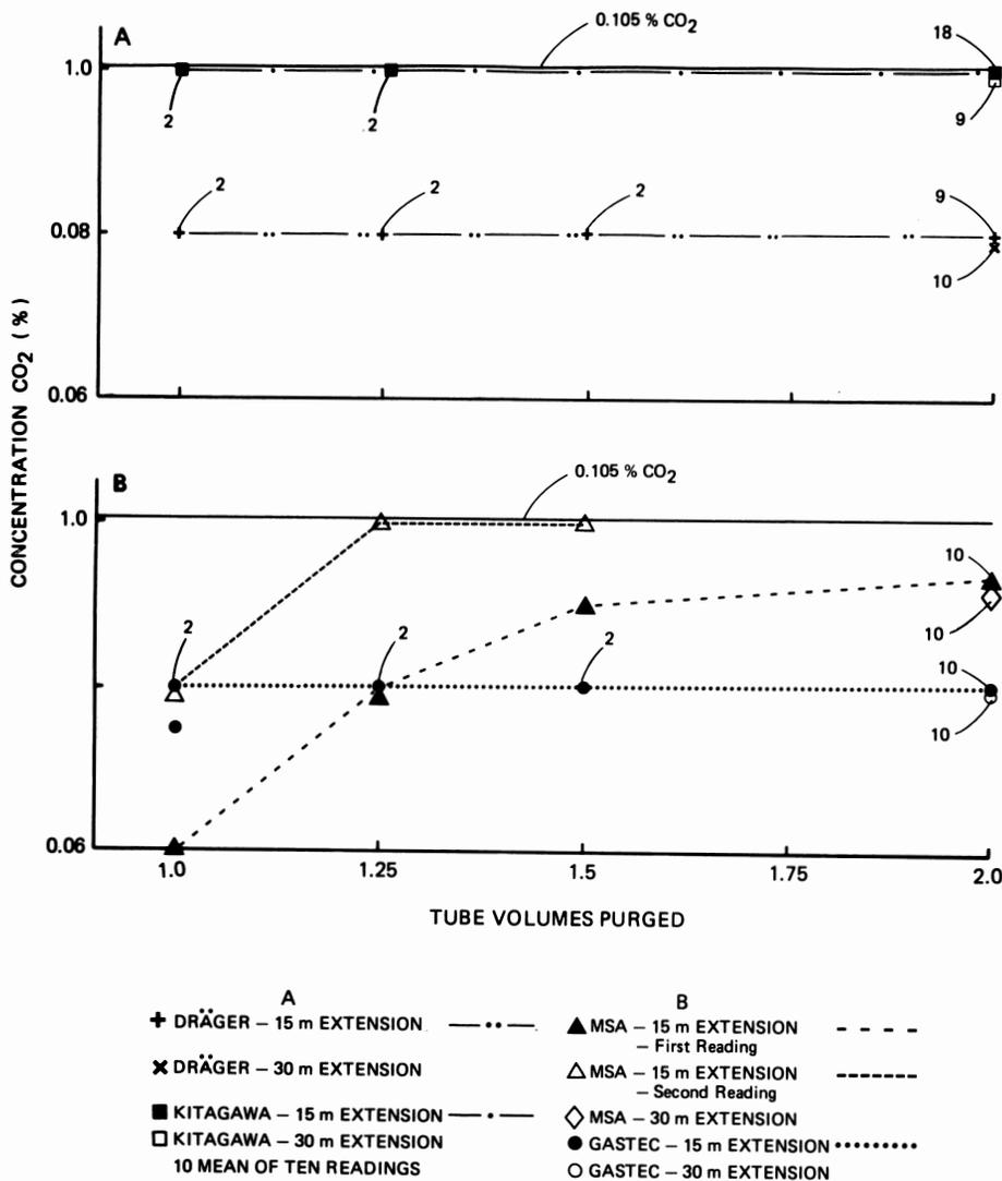
**Figure 10.** Effect of purge volume on remote detector accuracy. The test configuration was pump, detector tube, extension (15 or 30 m).
