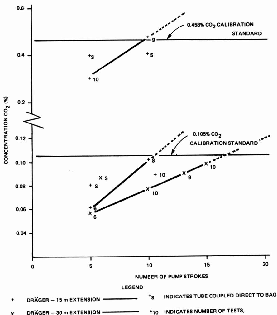
**Figure 11.** Effect of number of pump strokes on detector accuracy. The test configuration was pump, extension (15 or 30 m), detector tube.
