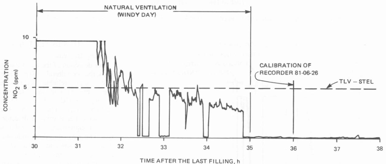
Figure 6. Recorder chart for  $\text{NO}_2$ , silo 23, 1981.
