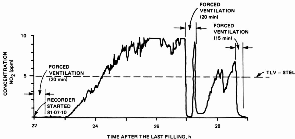
Figure 8. Recorder chart for NO<sub>2</sub> in silo 26, ventilated with a forage blower and 5-m drop tube, 1981.
