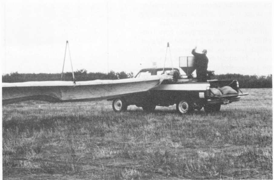
Figure 3. Truck-mounted bran spreader with shroud added. Note the effect of wind on the sides of the shroud, which are beginning to form an airfoil shape.
