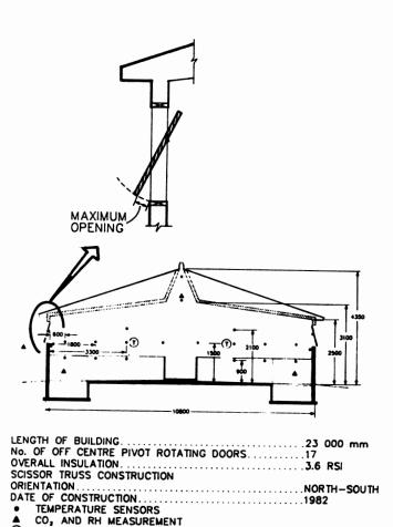
Fig. 1. Cross-section of barn showing location of thermocouples, and CO<sub>2</sub> and RH measurements.
