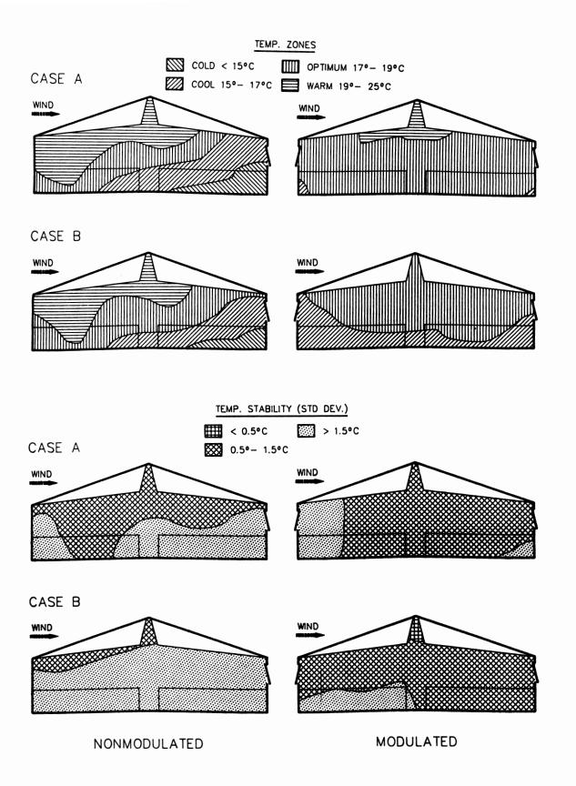
Fig. 3. Temperature zones, based on average temperatures over 1-h periods, and stability at a central cross-section of the barn for a modulated vs nonmodulated control system; Cases A and B represent exterior temperatures of approximately -3° and -11° C respectively; further details on exterior temperature and wind conditions are given in Fig. 2.
