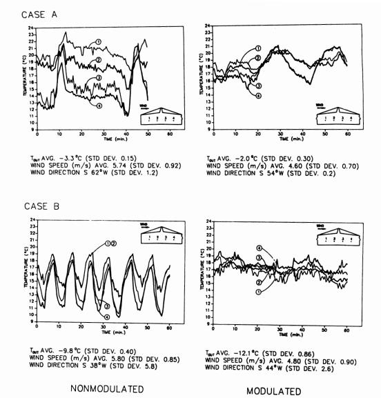
Fig. 2. Temperature variations at several locations near animal level using the modulated vs nonmodulated control system; the upper and lower figures represent results for exterior temperatures, T<sub>out</sub>, of approximately -3°C (Case A) and -11°C (Case B) respectively.
