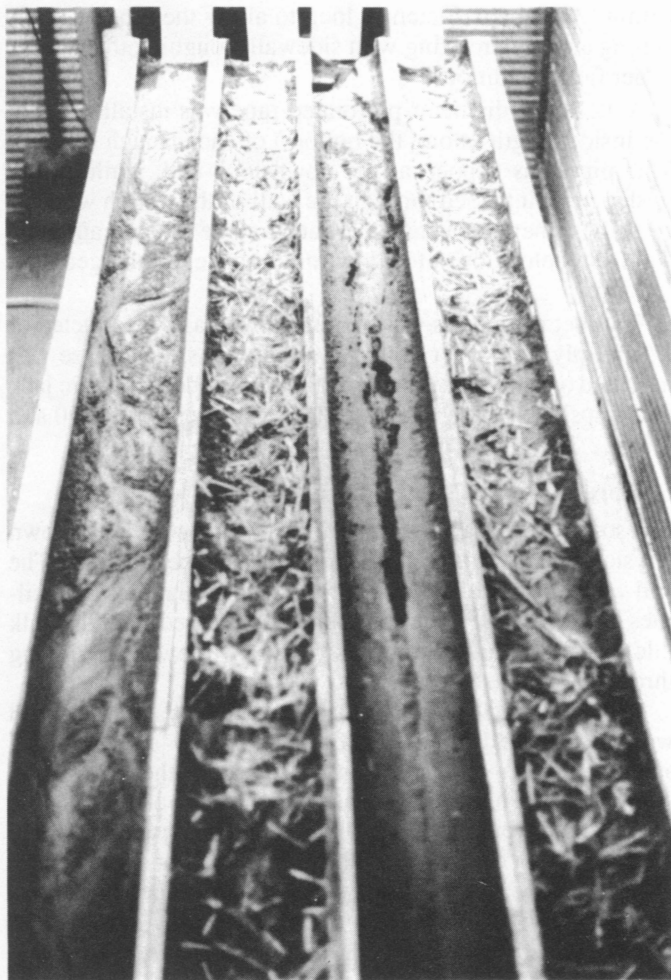
Fig. 3. Rills developed in troughs at end of a set of test runs, looking downslope.
