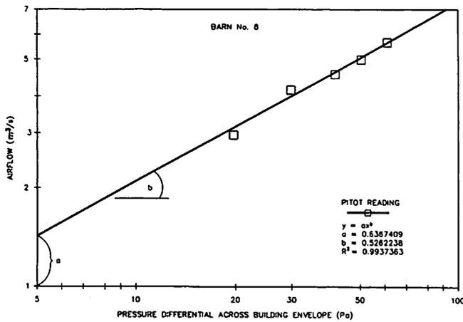
Fig. 3. Typical log-log plot of air flow versus pressure difference across the building envelope for a farm building.
