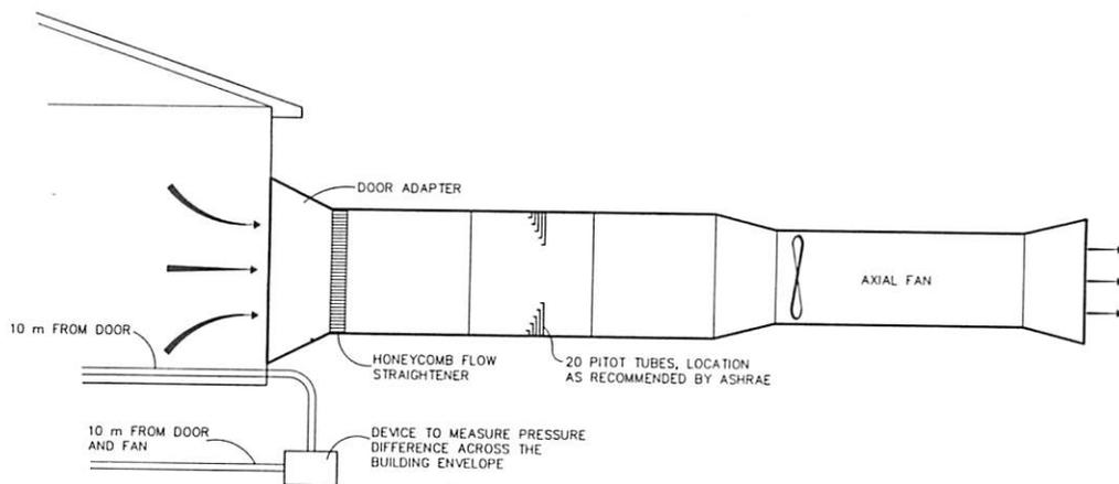
Fig. 1. Schematic diagram of the testing system.
