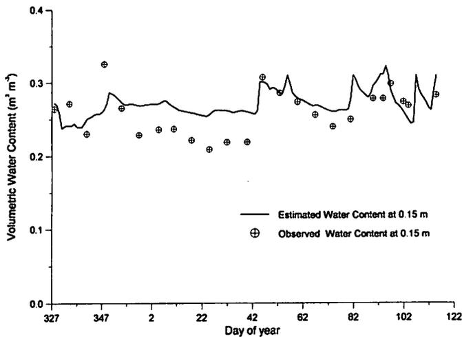
**Fig. 5. Model estimates of volumetric water content at the 0.15 m depth as compared to observed values measured with the TDR at the snow covered site.**
