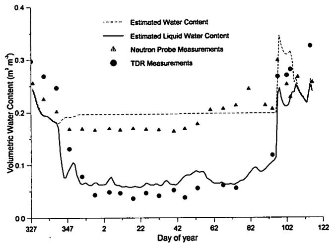
**Fig. 7. Model estimates of total volumetric water content and unfrozen water content at the 0.4 m depth as compared to observed values measured with the neutron probe and the TDR at the snow cleared site.**
