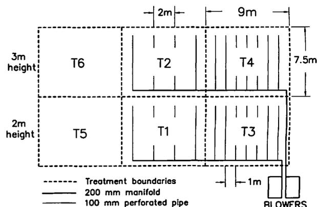
Fig. 1. Plan view of the experimental setup and abbreviations for the six aeration treatments.
