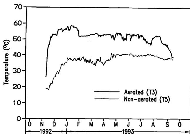
Fig. 3. Variations of temperature for an aerated and a non-aerated treatment.
