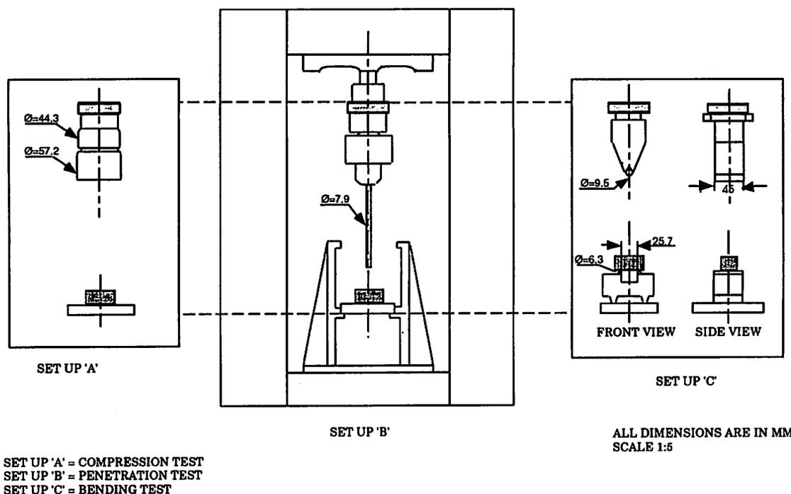
**Fig. 2. Schematic diagram of the set ups used in compression studies.**
