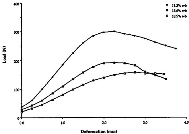
Fig. 5. Average load deformation curves for penetration tests on large cubes at different moisture contents.
