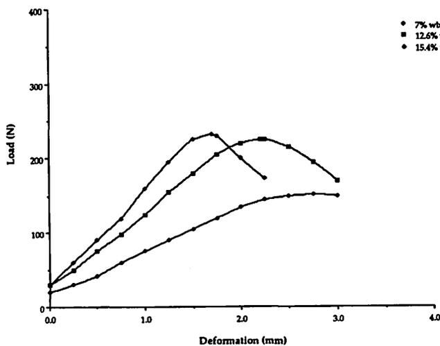
**Fig. 3. Average load deformation curves for penetration tests on regular cubes at different moisture contents.**
