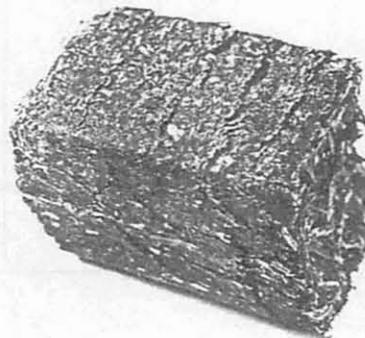
Fig. 1. A regular alfalfa cube with a cross section of 35 x 35 mm.
