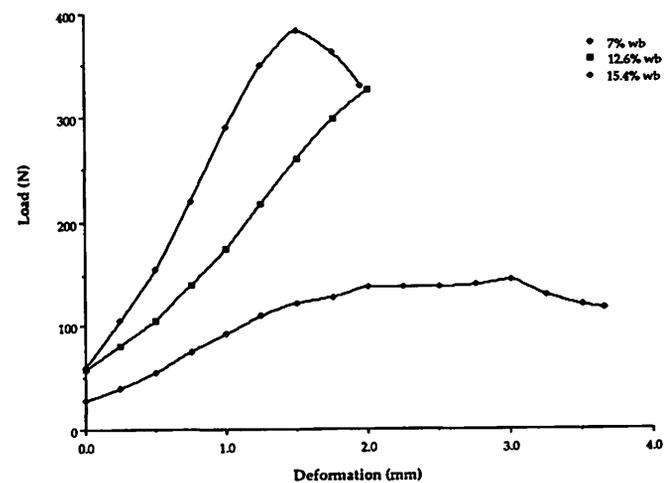
**Fig. 4. Average load deformation curves for bending tests on regular cubes at different moisture contents.**
