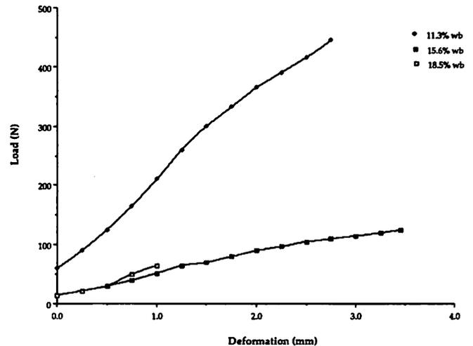
Fig. 6. Average load deformation curves for bending tests on large cubes at different moisture contents.
