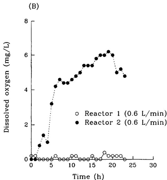
**Fig. 5. Dissolved oxygen levels of egg processing wastewater at aeration rates (A) 0.2 L/min and (B) 0.6 L/min for both reactors 1 and 2.**
