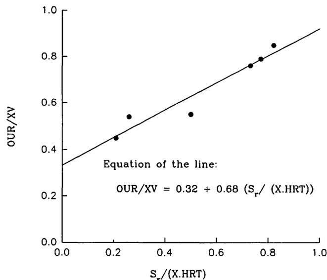
**Fig. 7. Determination of the aeration coefficients a' and b'.**
