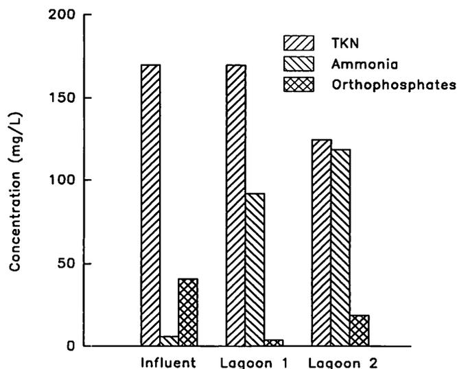
Fig. 4. TKN, ammonia, and orthophosphate values for egg processing wastewater treated by aerated lagoons.
