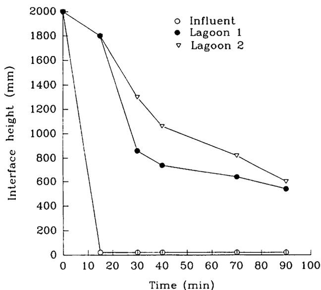
Fig. 3. Interface settling curves for egg processing wastewater in the aerobic lagoons.
