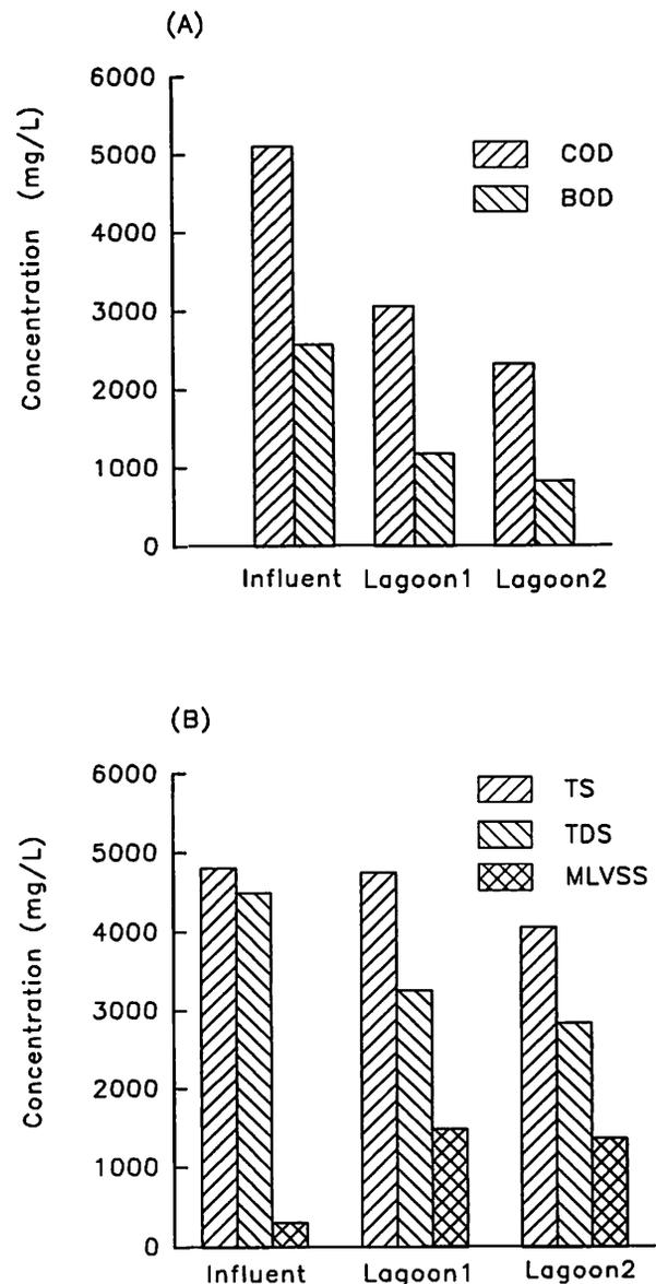
**Fig. 2. Reductions in (A) BOD, COD, and (B) solids in egg processing wastewater treated by an aerated lagoon system.**
