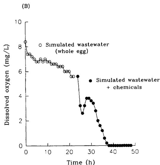
Fig. 8. Dissolved oxygen levels of (A) egg processing wastewater and (B) simulated egg processing wastewater and sanitary chemicals over time.
