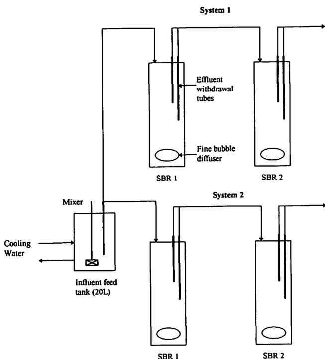
**Fig. 1. Process flow for the lab-scale 4L sequencing batch reactor system.**
