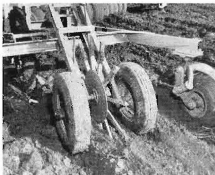
Figure 2. Spoke and surface sensing wheels of the depth transducer.
