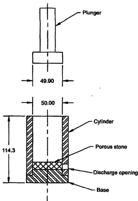
**Fig. 1. Schematic diagram of piston cylinder used for pressing alfalfa chops.**
