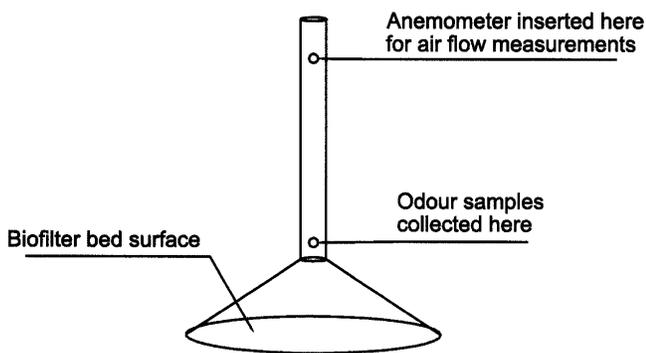
Fig. 3. Airflow sampling hood.
