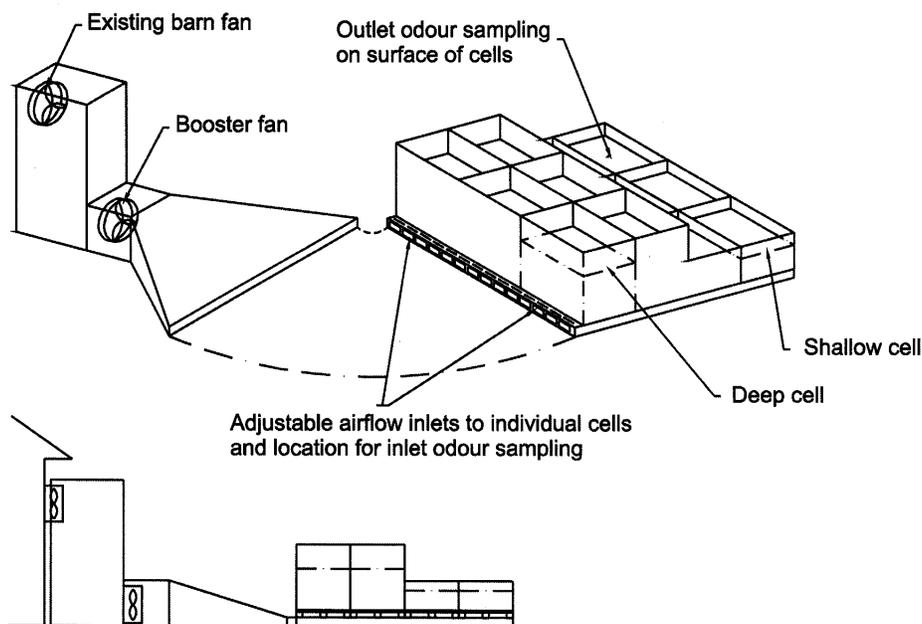
Fig. 2. Experimental biofilter configuration.
