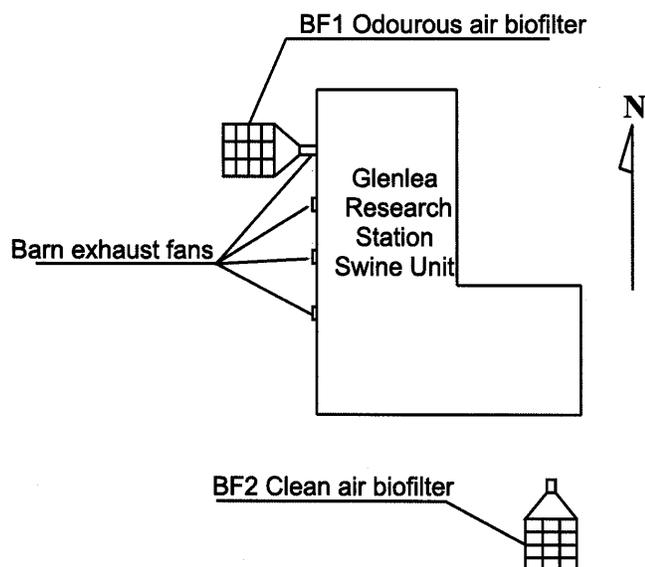
**Fig. 1. Layout of the two experimental biofilters in relation to the swine unit at the University of Manitoba Glenlea Research Station.**
