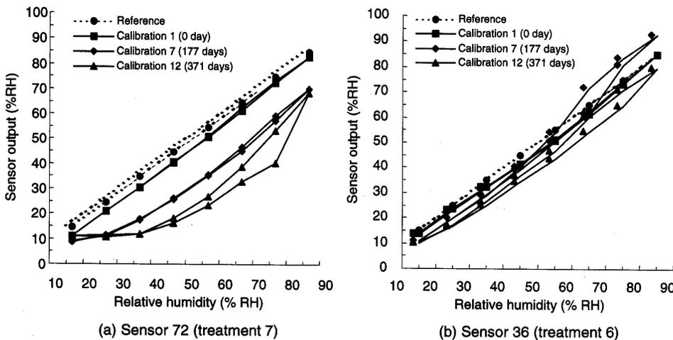
**Fig. 6. Accuracy drift of a treated and an untreated sensor over the year.**
