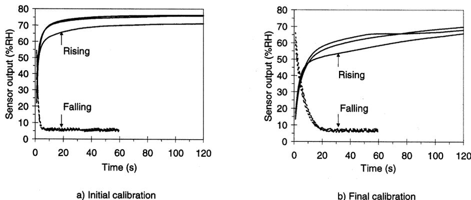
**Fig. 7. Output of sensor 36 for the initial and final time response calibration.**
