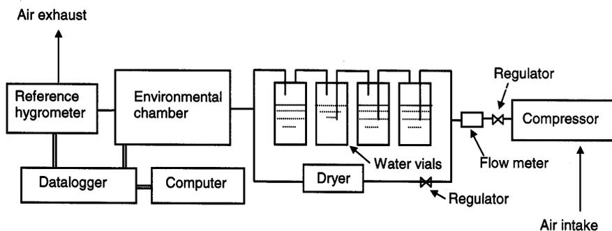
**Fig. 1. Schematic diagram of the calibration equipment.**
