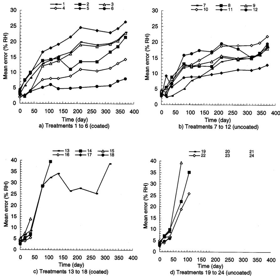
Fig. 5. Accuracy drift of CHS-UGS and CHS-GSS sensors over the year.
