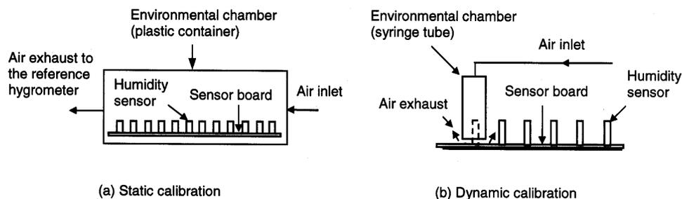
**Fig. 3. Sectional sketch of environmental chambers for static and dynamic calibrations.**
