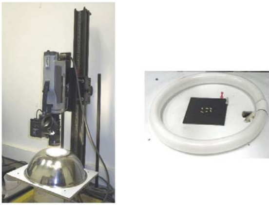
Fig. 1. Image acquisition system (left) and illumination system (right).
