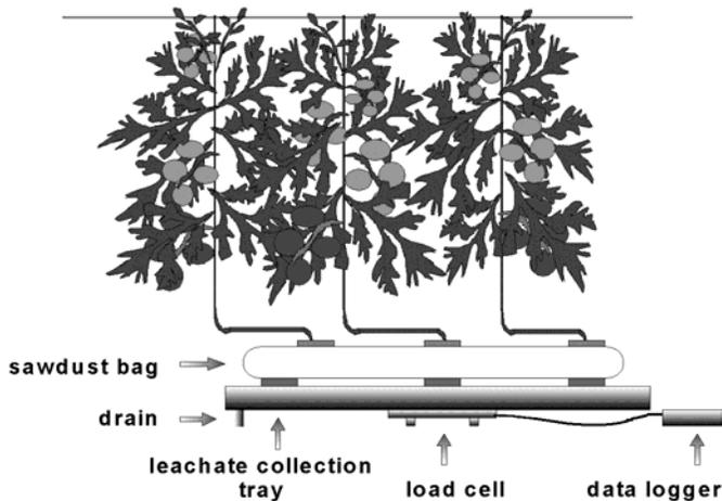
Fig. 1. Layout of equipment utilized in the weight-based control algorithm.
