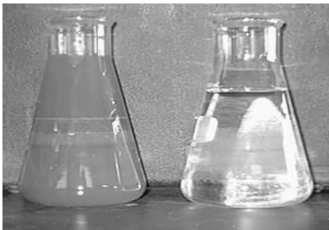
Fig. 3. Picture of liquid manure before and after RO filtration.
