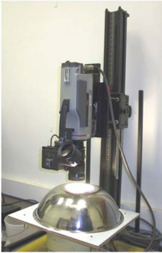
Fig. 1. Image acquisition setup and a representative image of bulk Canada Western Amber Durum wheat.
