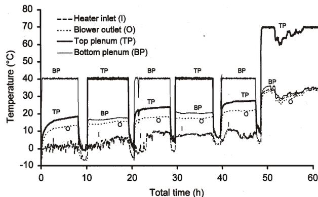
**Fig. 6. Air temperature at four positions in the dryer as a function of total time for experiment #1 (9-bale batch). Airflow was interrupted and direction reversed five times after every 8-h period with about 1 h interruption for bale weighing. Inlet air was ambient except in the sixth drying period when about 89% exhaust (outlet) air was recirculated.**
