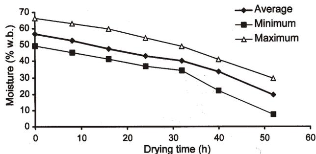
**Fig. 5. Moisture content (wet basis) of corn stover bales during drying experiment #1 (9-bale batch on one layer 0.89 m high). Values are based on average DM from initial and final moisture content samples and mass balance for each bale.**
