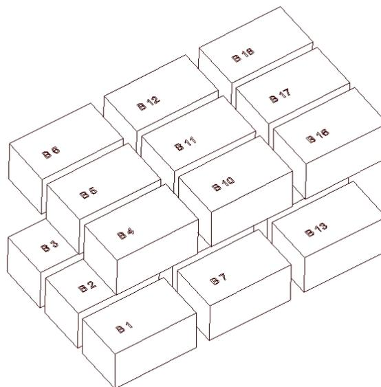
**Fig. 3. Schematic view of placement of two layers of corn stover bales in dryer as in experiment #2.**
