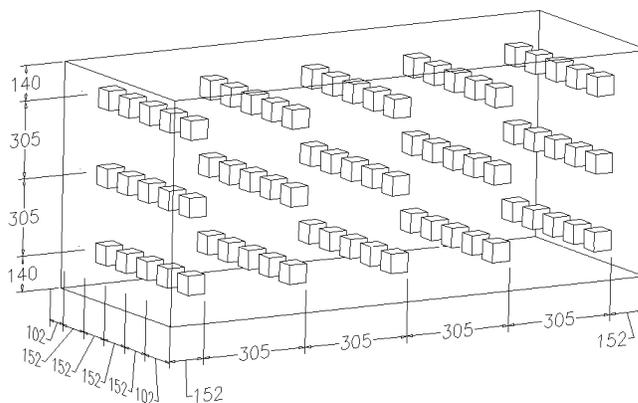
**Fig. 4. Schematic view of 75 samples cut out from selected bales to estimate moisture content variation after drying and storage. Dimensions are in millimeters.**
