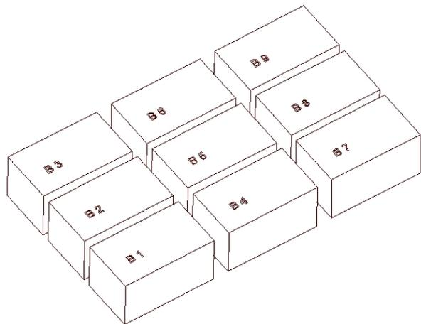
**Fig. 2. Schematic view of placement of one layer of corn stover bales in dryer as in experiment #1.**
