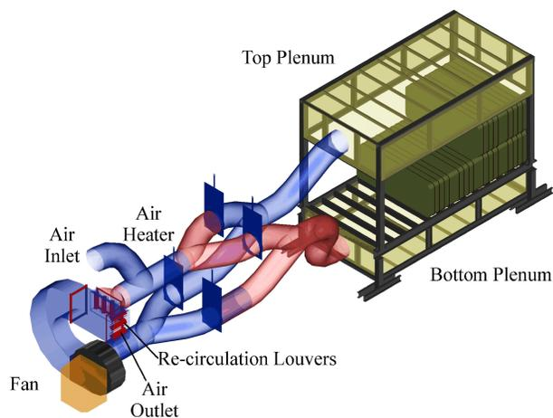
**Fig. 1. Schematic view of the bale dryer with bi-directional airflow.**
