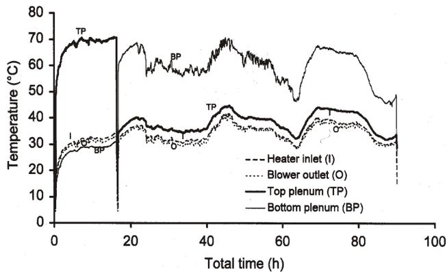
**Fig 7. Air temperature at four positions in the dryer as a function of total time for experiment #2 (18-bale batch). Airflow was interrupted and direction reversed once after 16 h of drying. Inlet air was composed of about 89% recirculated outlet air and 11% ambient air.**
