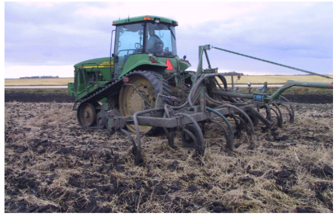
Fig. 3. Field injection unit with 13 narrow sweeps in two ranks (seven sweeps in the first rank and six sweeps in the second rank).
