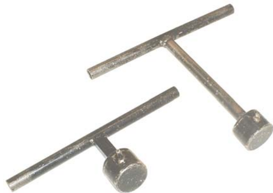
Fig. 2. Core sampler of 73 mm diameter (circled) used with a standard handle for 0 - 180 mm depth or an elongated handle for 180 - 360 mm depth.
