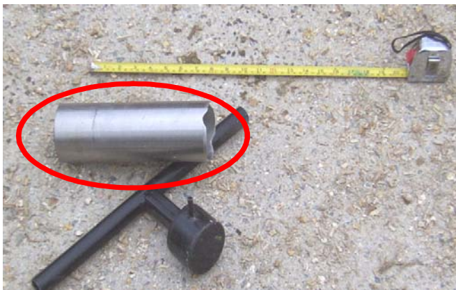
Fig. 2. Core sampler of 73 mm diameter (circled) used with a standard handle for 0 - 180 mm depth or an elongated handle for 180 - 360 mm depth.
