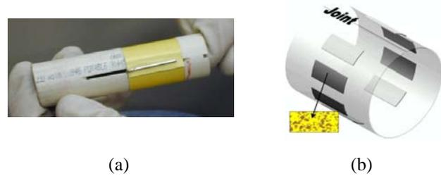
**Fig. 4. (a) Strip of water-sensitive paper wrapped around a tube with the metal clip inserted. (b) Location of the image around a single sampling tube (to scale) and a sample image.**
