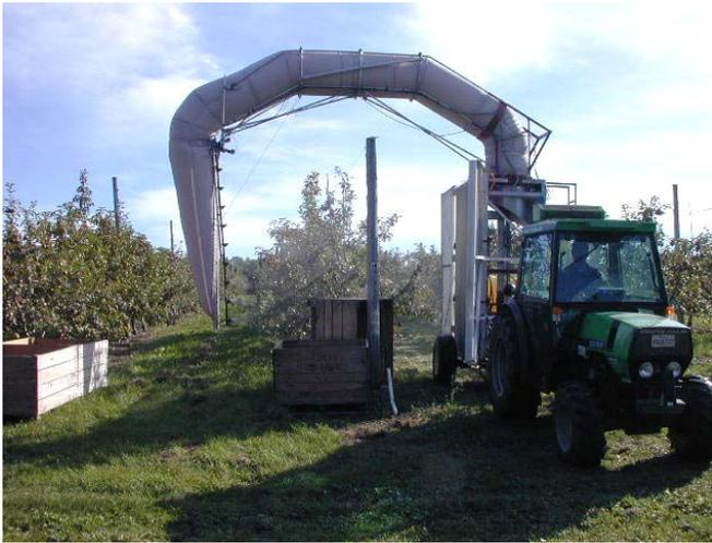
**Fig. 1. RÉCUPAIR sprayer for orchard – spray recovery sprayer (SRS).**
