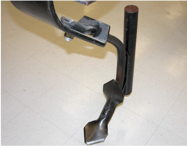
Fig. 4. Close-up of the 108-mm wide reversible mulch sweep used on the Kongskilde field cultivator.
