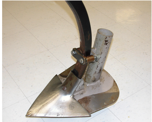
Fig. 6. Husky injector fabricated from a 304-mm wide sweep and fitted with a rear cover plate and drop tube.
