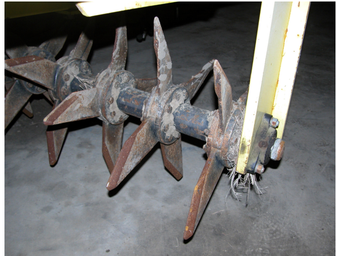
Fig. 2. Close-up of roller on AerWay® soil aerator showing arrangement of tines bolted to hubs on the roller axle.
