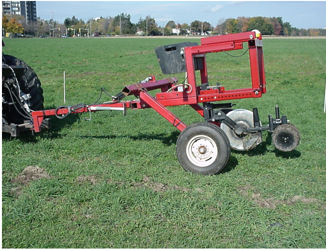
Fig. 8. Instrumented toolbar for measurement of single injector draft. The toolbar is suspended on a parallel arm linkage to isolate extraneous forces and moments from draft force acting on the injector.
