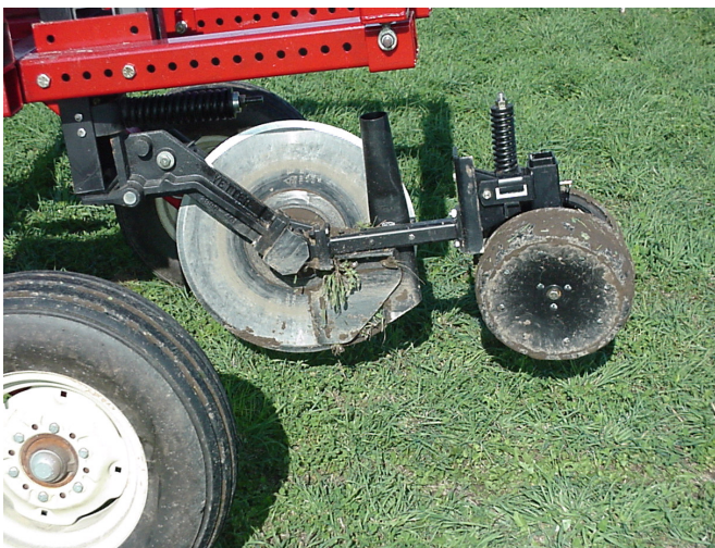
Fig. 5. Yetter single disk injector. Manure is deposited via the drop tube located between the stationary shoe and the disk. The furrow is closed with the rear press wheels.
