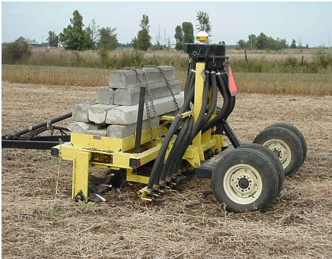
Fig. 1. AerWay® soil aerator (3.1 m wide) fitted with SSD manure application kit including distributor and drop tubes. Concrete parking curbs were used as ballast to ensure adequate penetration in hard soil. The machine is operating in soybean residue at site 3.
