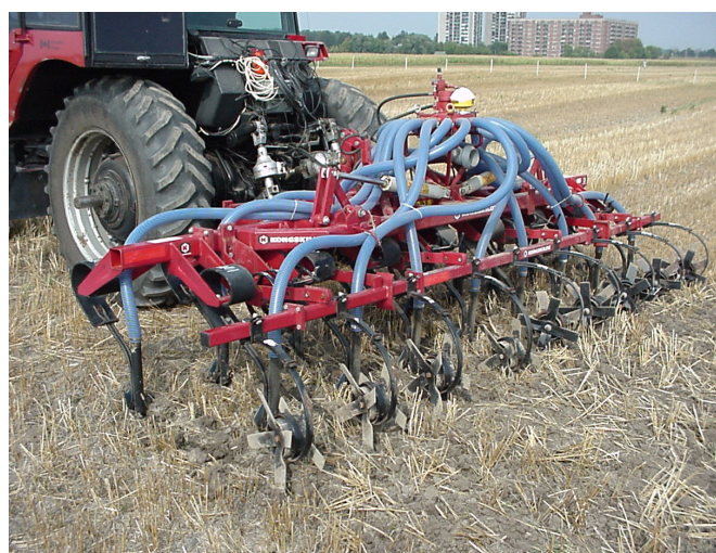
Fig. 3. Kongskilde field cultivator (4.7-m wide) with 17 Vibro-Flex shanks spaced at 275 and 108-mm wide mulch sweeps. The unit was fitted with a distributor and drop tubes for manure application. The machine is operating in barley stubble at site 2.
