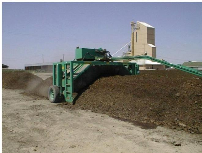
**Fig. 2. Earthsaver CT-12 windrow turner used to turn the windrows.**
