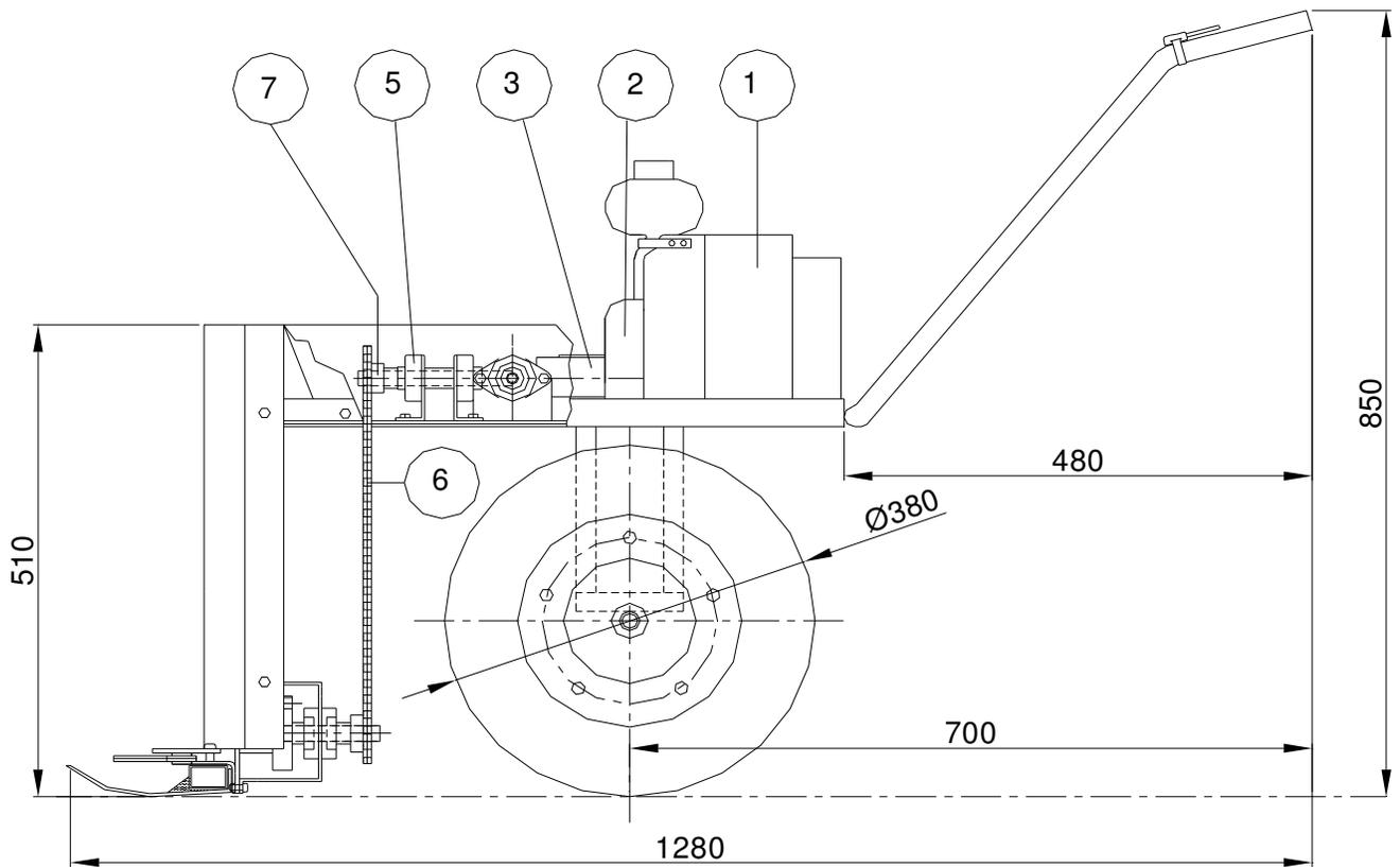
Fig. 3. Side view of the cutter bar mower (dimensions in millimeters)
