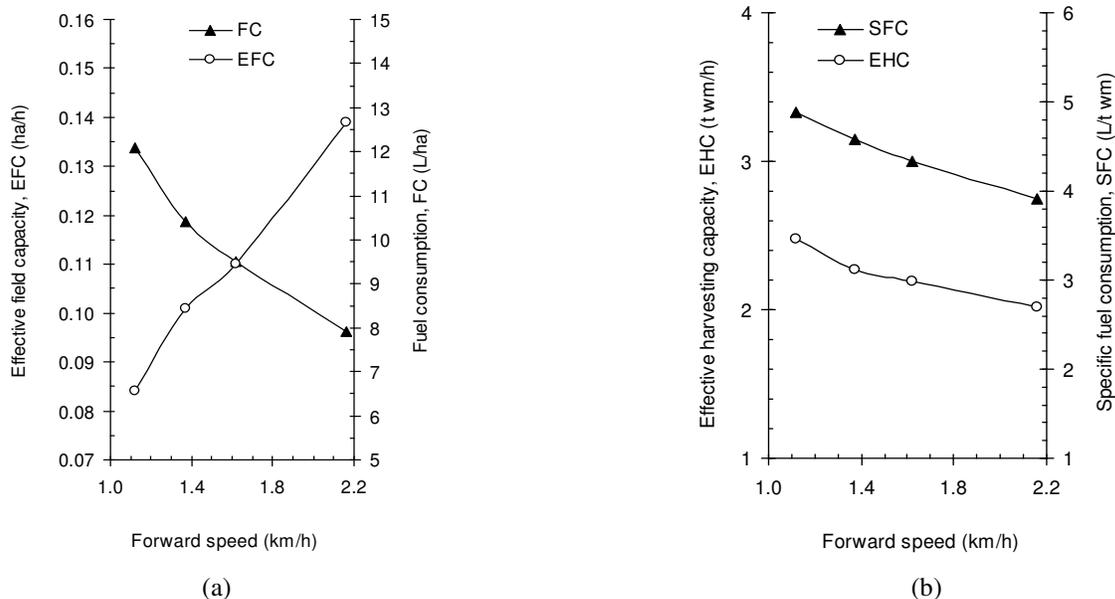
**Fig. 4. (a) Effective field capacity and fuel consumption vs forward speed; (b) Effective harvesting capacity and specific fuel consumption vs forward speed.**
