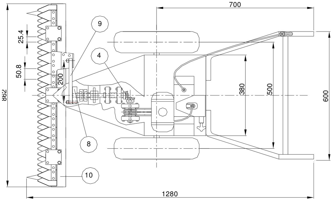
Fig. 2. Top view of the cutter bar mower (dimensions in millimeters).
