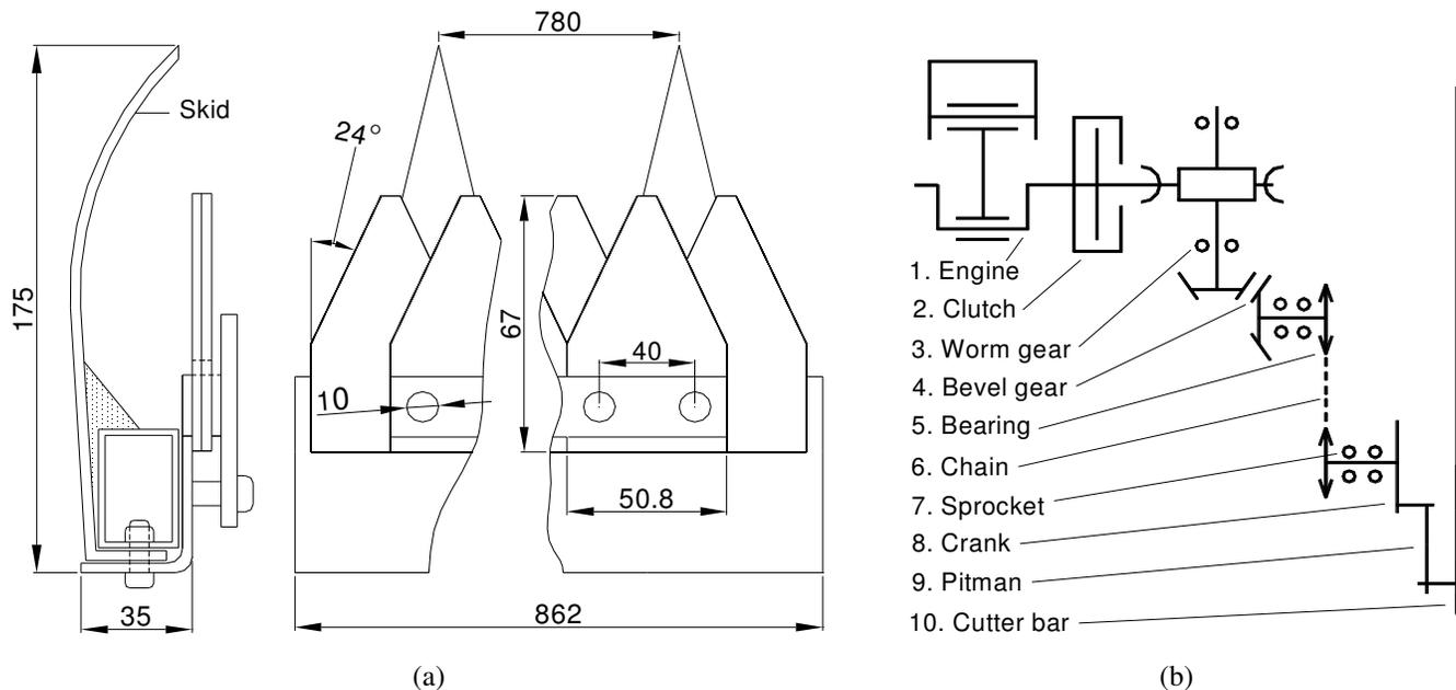
**Fig. 1. (a) Dimensions (millimeters) of knife and skids (left side view and top view); (b) Diagram of the mechanical elements of the transmission unit.**
