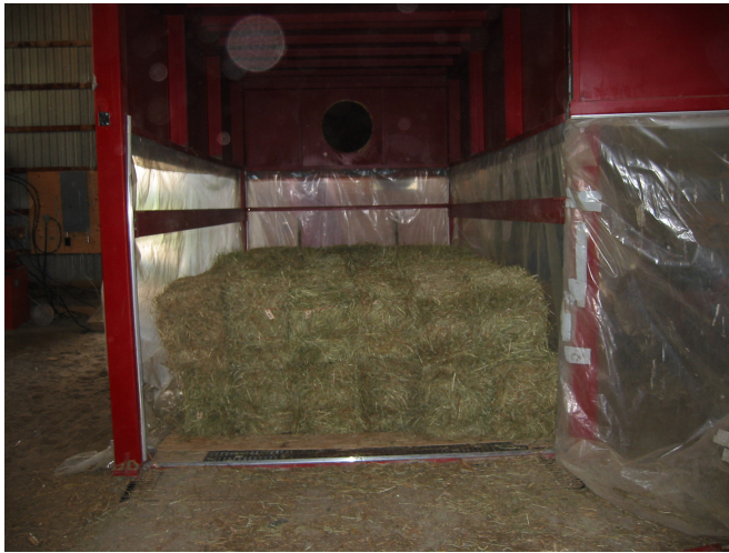
Fig. 3. Drying chamber with 60 small hay bales over two levels between the upper and lower plenums. Door is closed and polyethylene adheres to bales during drying under suction.
