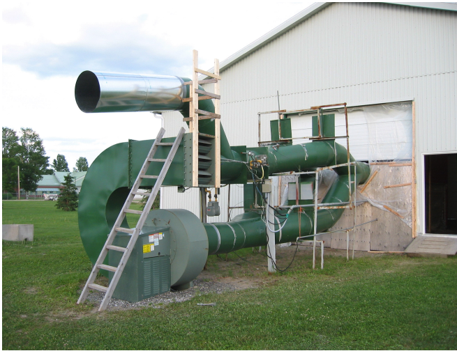
Fig. 1. Air flow system with propane gas burner, four gate valves for directional change, blower pulling air in negative pressure, and two louvers to control recirculation.
