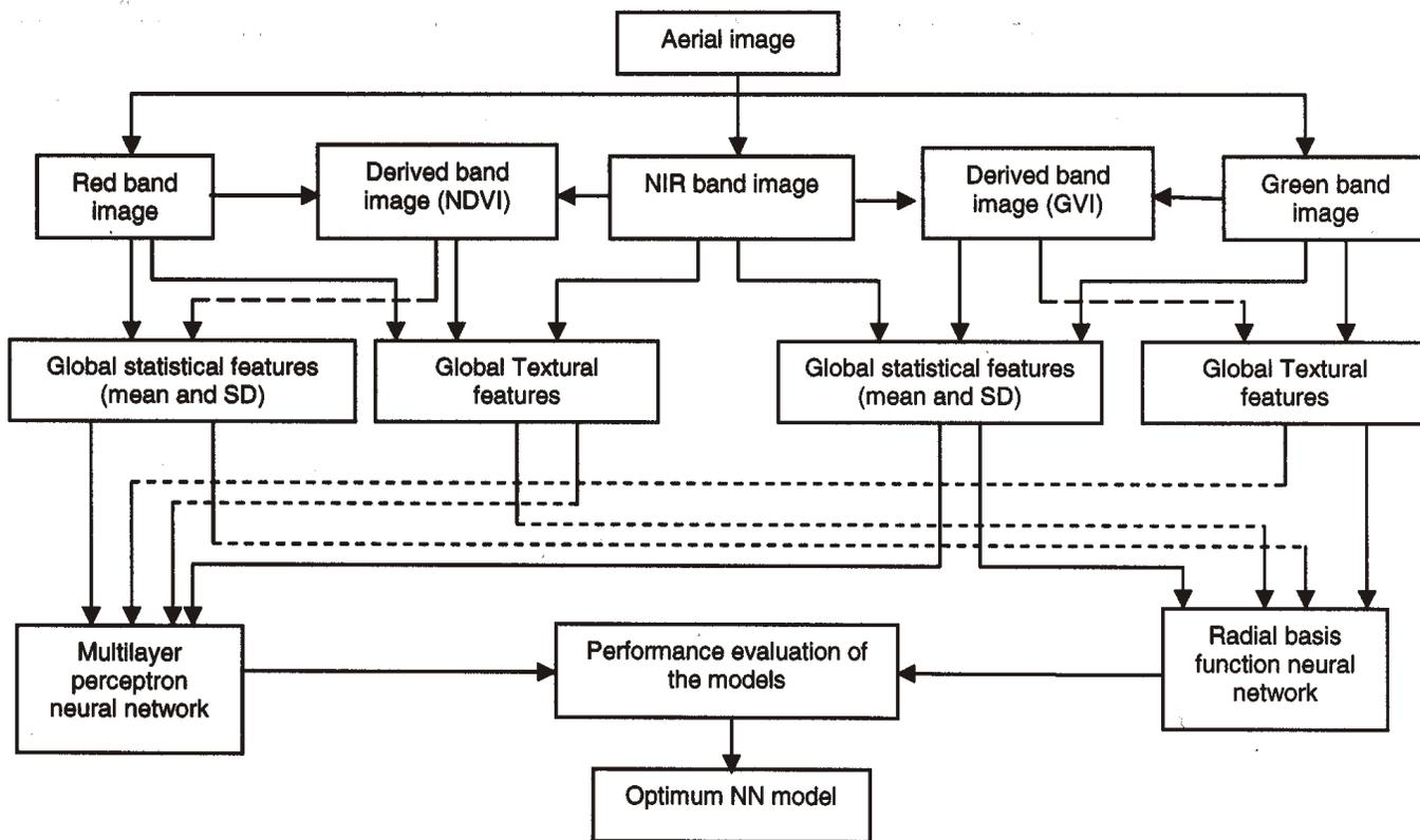
**Fig. 1.** Overall process involved to determine an optimal NN model from a set of potential neural network models for predicting leaf nitrogen content using aerial images under field conditions.
