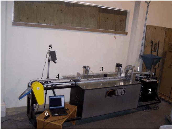
**Fig. 1. Experimental setup. 1 - grain inlet, 2 - control panel, 3 - microwave chamber, 4 - conveyor, 5 - thermal camera, 6 - data acquisition system**
