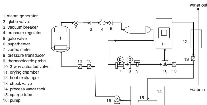
Fig. 2. Schematic of the superheated steam processing system.
