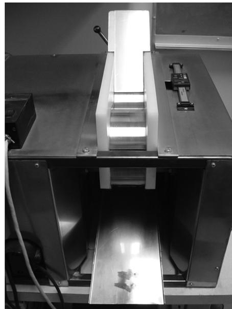
Fig. 1. Laboratory noodle sheeter (75 mm wide rolls).
