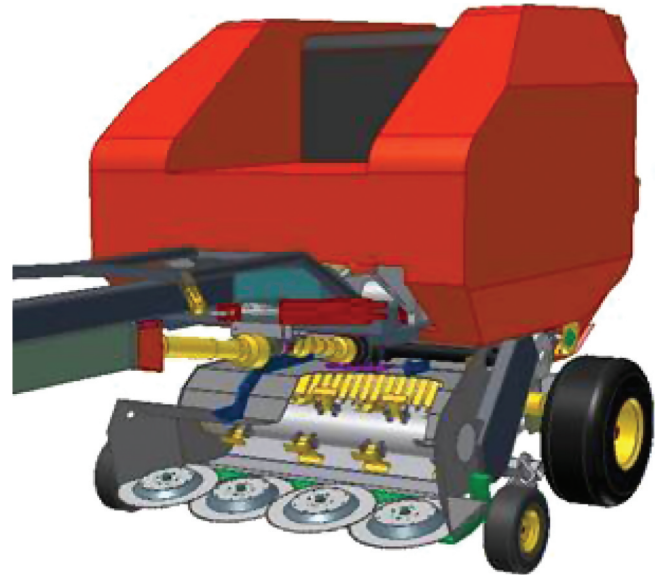
Fig. 1. Original four-saw cutter head developed to harvest willow plantations on level land.
