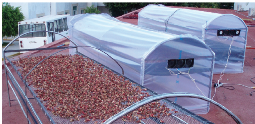
Fig. 1. Chamber used for roselle drying.
