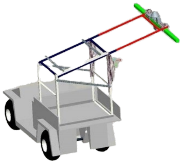
Fig. 1. Vehicle-based laser system for surface microtopography measurement.
