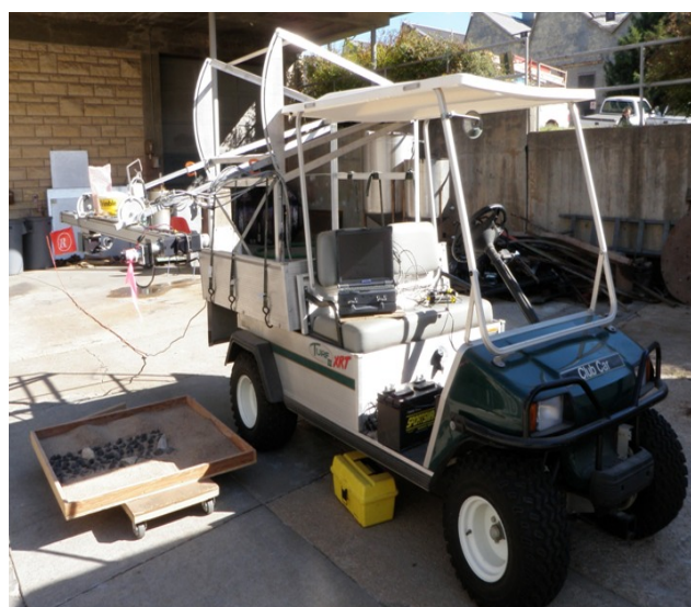
Fig. 4. The vehicle-based laser system measures the DEM of the test surface.
