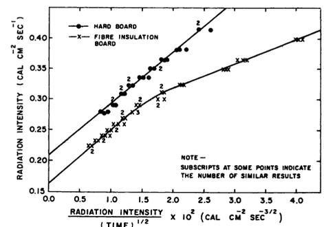
Figure 2. Pilot Ignition of Fibre Boards.
