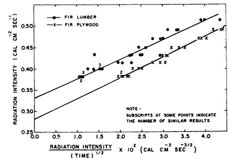
Figure 1. Pilot Ignition of Plywood and Fir.
