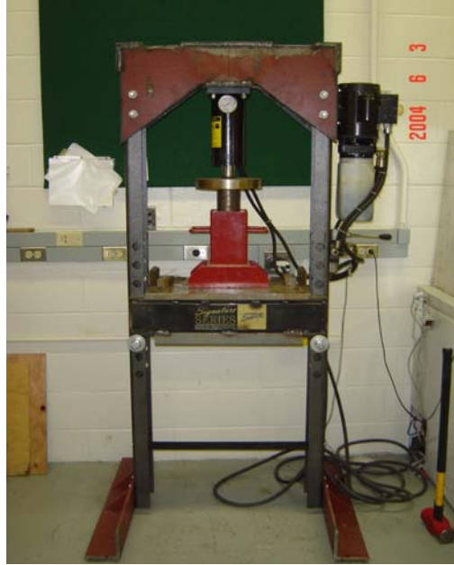
Fig.1. The hydraulic press used for compressing hays.
