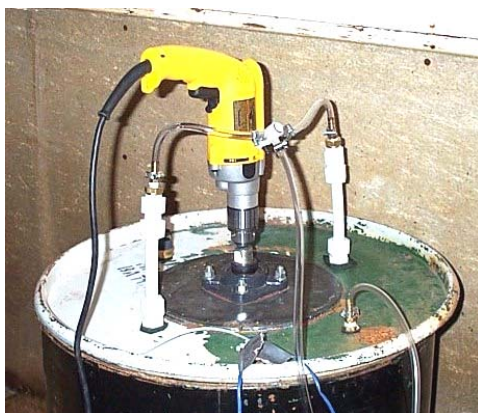
Figure 3. Modified barrel lid to allow agitation and spray, and sampling of headspace gases.
