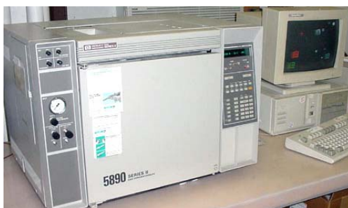
Figure 4. GC system used as reference method for determining H 2 S levels in gas samples.
