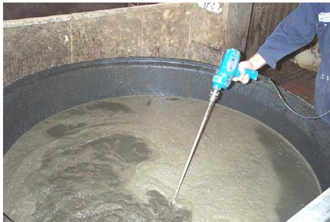
Figure 2. Mixing the manure sample in the large tub prior to filling the barrels.
