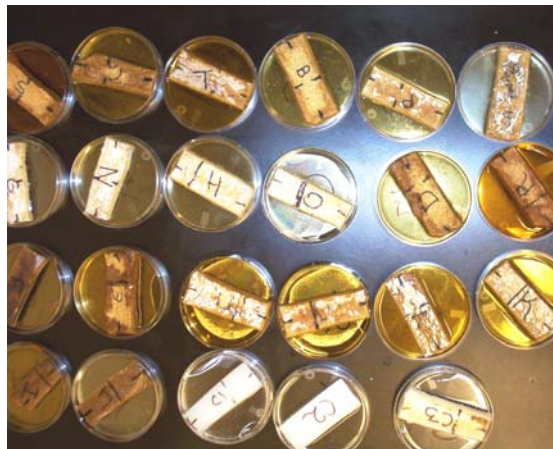
Figure 1. Water absorption testing of biocomposite samples.
