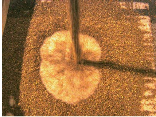
Figure 3. Ring formed due to grain impact with grain chamber bottom.
