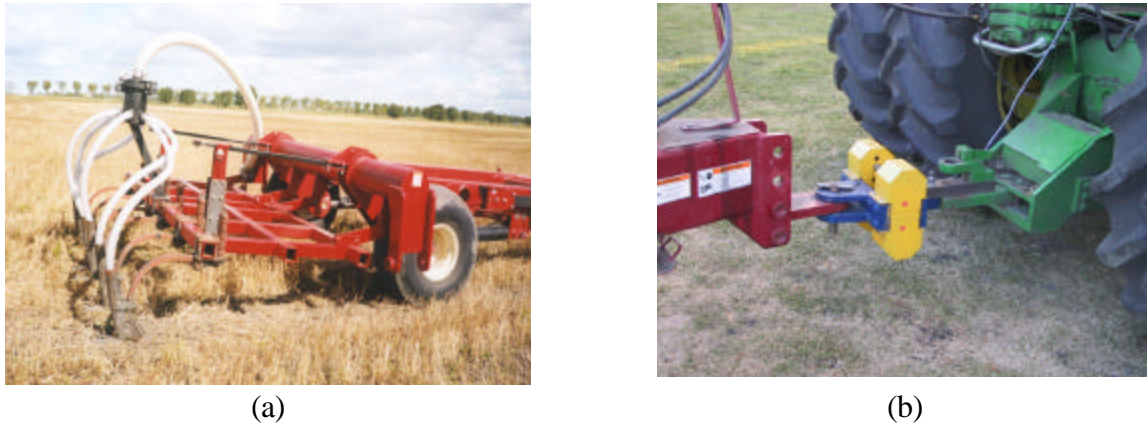
Fig. 6. Equipment used for the field tests; (a) liquid manure injector with six sweep-type tools; (b) DEOR dynamometer installed between the tractor and the injector hitch to measure the drawbar forces.
