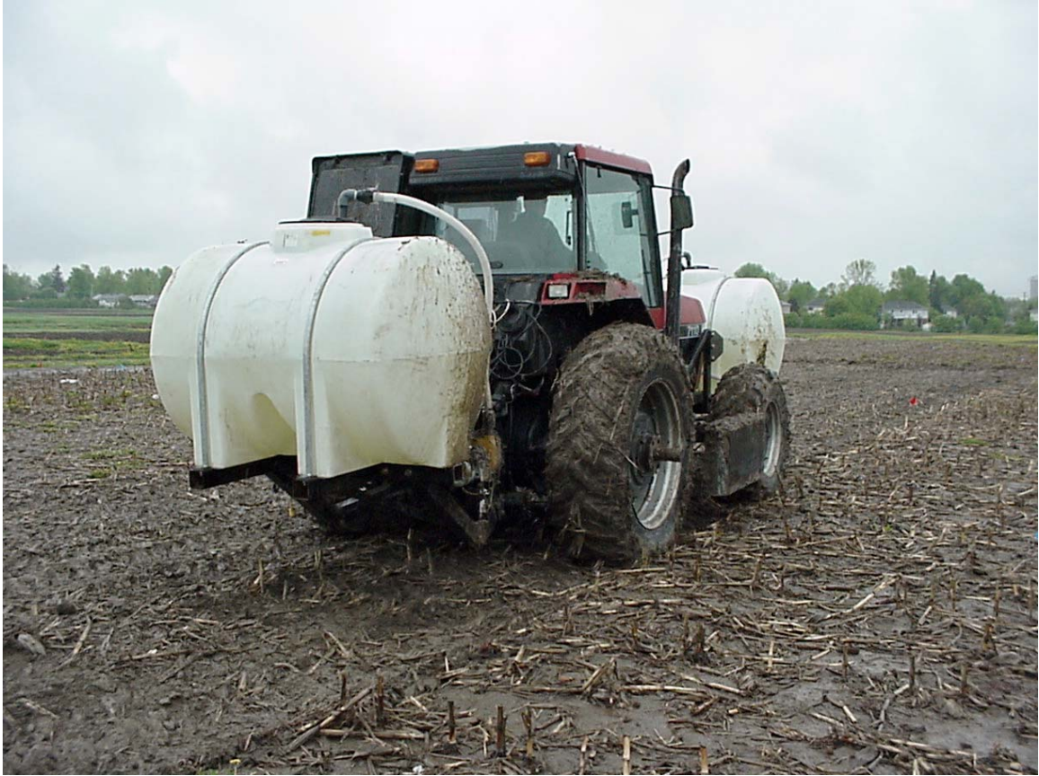
Fig. 2 Tractor used to compact plots in a wheel-beside-wheel manner. The large tanks mounted on front and rear of the tractor were each filled with 2000 litres of water for increased ballast. Total tractor mass including water ballast was about 14 Mg.
