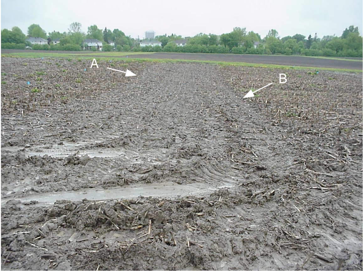
Fig. 5. Photograph of compacted plot. The A and B arrows point to the border between the compacted plot and adjacent non-compacted plots. Note rutting and skidding in foreground at the bottom of the photograph resulting from turning the tractor in the buffer zone between reps 3 and 4 and reps 1 and 2 (Fig. 3).
