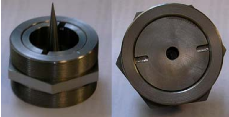
Figure 3.1: Assembled cartridge; Left - inlet of cartridge; Right - outlet of cartridge
