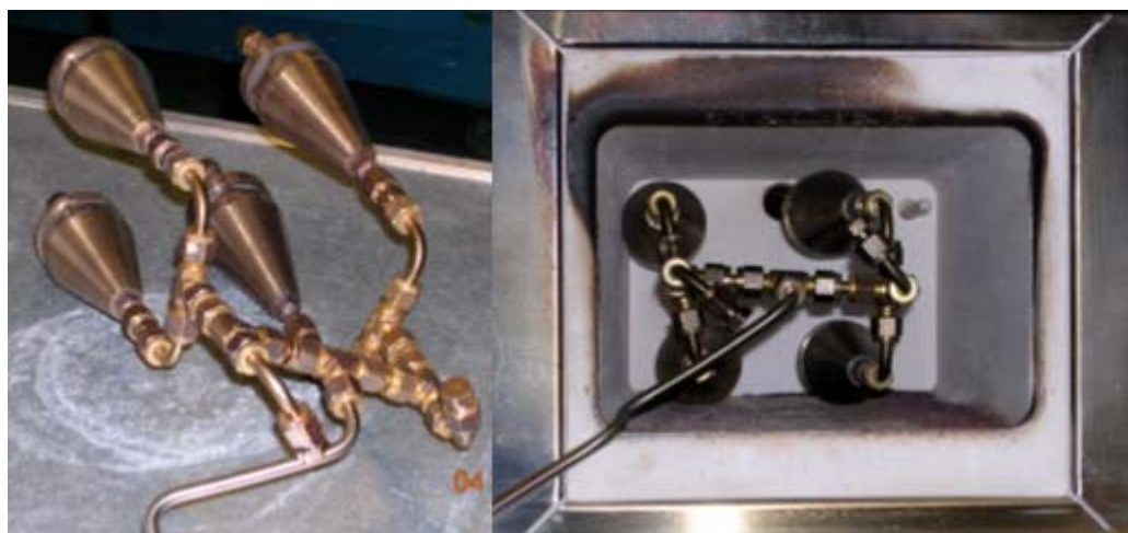
Figure4.1: Left; Sampler connected to piping to deliver N 2 to sampler during conditioning. Right; Samplers and piping placed in the oven
