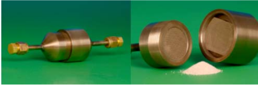
Figure 2.2: Photos of the sampler; Left: Complete sampler; Right: Opened sampler and zeolite molecular sieve 5A
