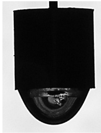
Figure 7. Photograph of a pendant drop, showing the calibration cylinder.
