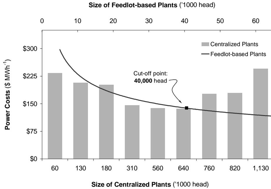
**Fig. 5.** Feedlot-based power cost vs. centralized processing in concentrated feedlot areas in the absence of digestate processing.
