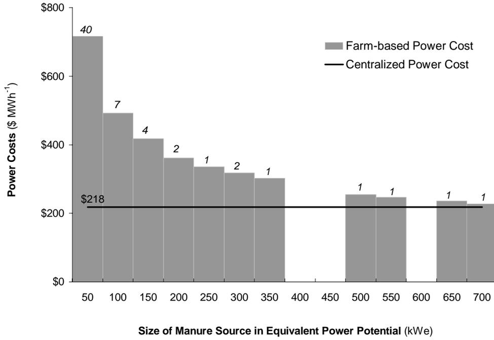
**Fig. 4.** Farm-based power cost as a function of capacity vs. centralized processing in Red Deer County (number of manure sources at each capacity is identified at the top of bar charts).
