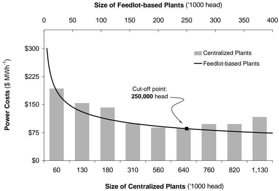
**Fig. 6.** Feedlot-based power cost vs. centralized processing in concentrated feedlot areas with subsequent digestate processing.
