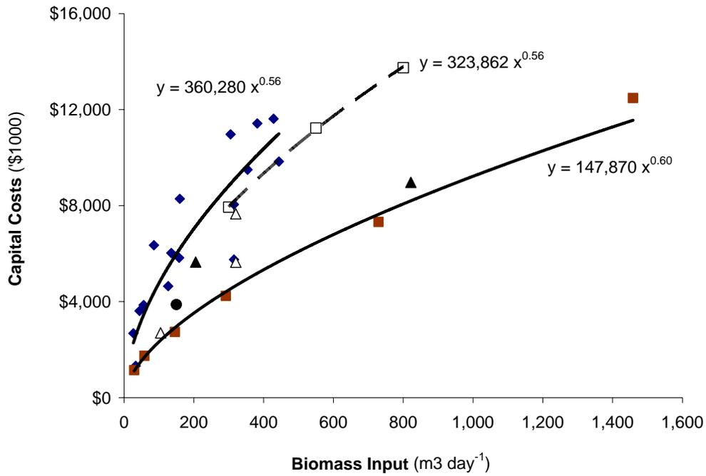
**Fig. 1.** The estimated cost of biogas plants generating electric power (■ Hashimoto et al. (1979); ● Mathony et al. (1999); ◆ H-Gregersen (1999); □ Nielsen and H-Gregersen (2002); ▲ Row and Neable (2005); △ Tofani (2006))
