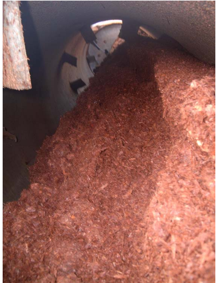
Photo 2, June 28, 2005: Interior view, desired level of the composter with 2/3 of the total capacity.
