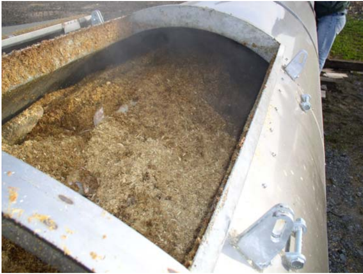
Photo 1, May 6, 2005: Opening # 1, entrance of the mortalities with wood shaving and recycled compost.
